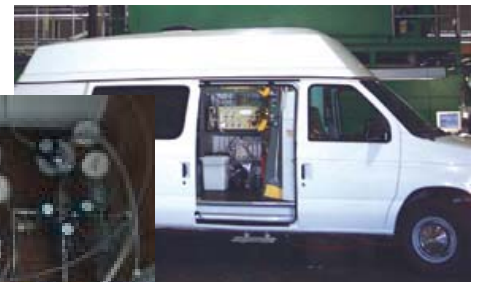
Chemists in the District's Monitoring Division use specially-equipped vans to sample emissions from industrial sources to make sure they do not exceed the limits specified on their air quality permits.
