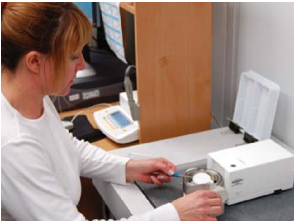
Particulate matter is monitored by capturing the tiny particles on filters and the concentration determined by their weight.
