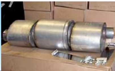
Retrofitting Mexico-based trucks that go back and forth across the border with a diesel oxidation catalyst (pictured above) cuts their emissions, thus helping to improve our air quality.
