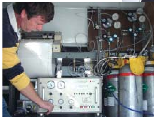
Chemists in the District's Monitoring Division use specially-equipped vans to sample emissions from industrial sources to make sure they do not exceed the limits specified on their air quality permits.
