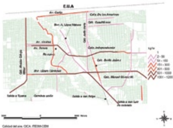
A sample of CO emissions in kilograms per hour was taken at 7 a.m. on different roadways in Mexicali (above). The photographs at right show Dzoara Tejeda's team setting up a system to monitor traffic flow with the help of local police.
