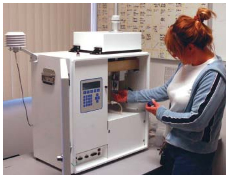
A District chemist loads a filter holder into a particulate sampler to prepare it for placement at a monitoring site.
