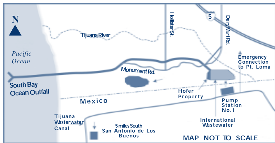
Map of the South Bay International Wastewater Treatment Plant project site. The South Bay ocean outfall that extends 3.5 miles offshore is scheduled for completion this Fall.
