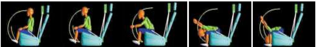
6-year-old child dummy, scooted forward in seat, restrained by the **lap belt only**. 35 mph crash. **Extensive dummy movement.**
