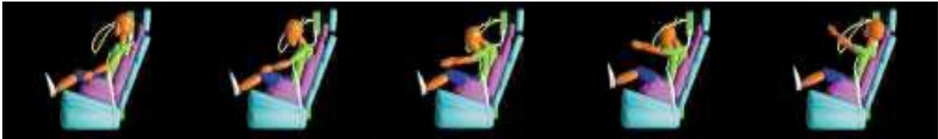
6-year-old child dummy in a belt-positioning **booster seat**, restrained by a lap-shoulder belt. 35 mph frontal crash. **Little dummy movement**
